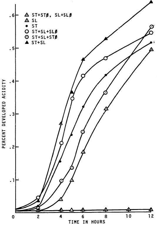
Figure 18. Effect of cellular lysis by bacteriophage ( $\emptyset$ ) on associative growth of <u>S</u>. <u>lactis</u> MS (SL) and <u>S</u>. <u>thermophilus</u> ST<sub>4</sub> (ST) strains as measured by acid production.
